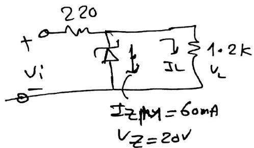
∴  $V_{in} = 23.67 \text{ V}$
