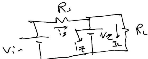
$$\rightarrow \because V_L = V_Z \quad \& \quad I_L = \frac{V_Z}{R_L}$$
