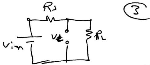
Now, if  $V_{in} < V_Z$   $\therefore$  Zener (off)  $\Rightarrow$  open &  $V_Z = \frac{V_{in} R_L}{R_L + R_S}, I_Z = 0$
